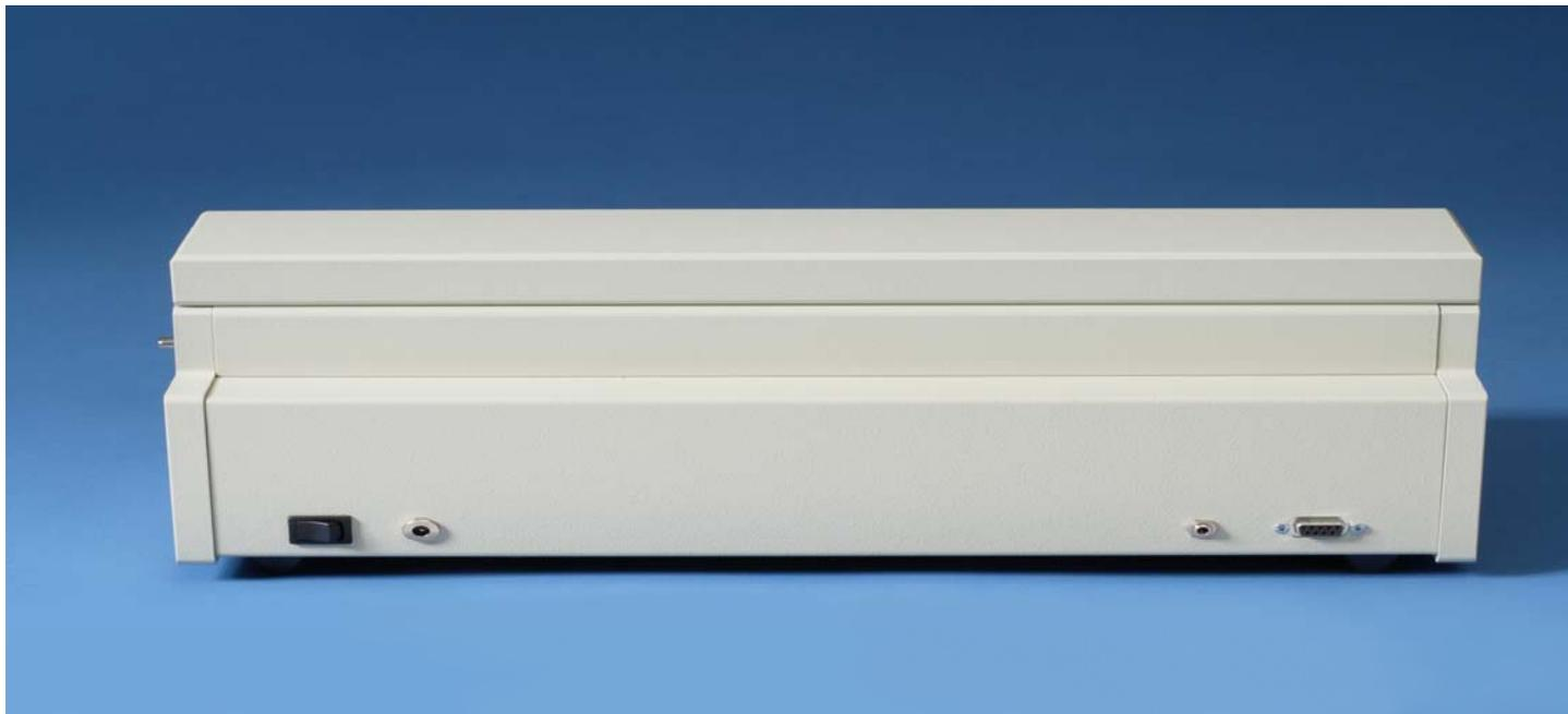
The rear panel of the CO50 has an ON/OFF switch, a DC power input jack for connecting the bench top power supply, a counter jack for connecting the injection counter, and an I/O port for the RS232. The I/O port will be discussed later in the chapter on the RS232. There is a reorder label on the rear panel that tells the model number, serial number, operating voltage of the unit, power consumption and the address information for Torrey Pines Scientific.
