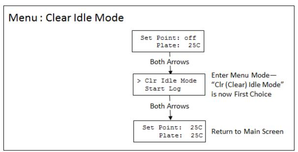
Figure 6: Menu Map to Clear Idle Mode Using the Menu
