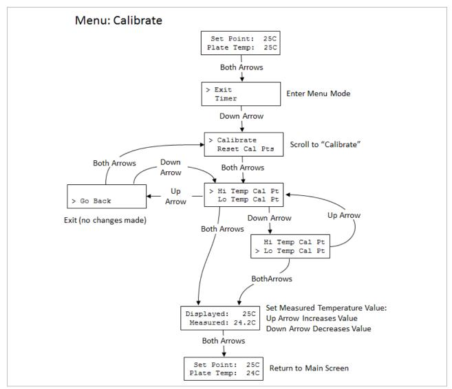
Figure 10: Menu Map to Calibrate the Plate Temperatures
