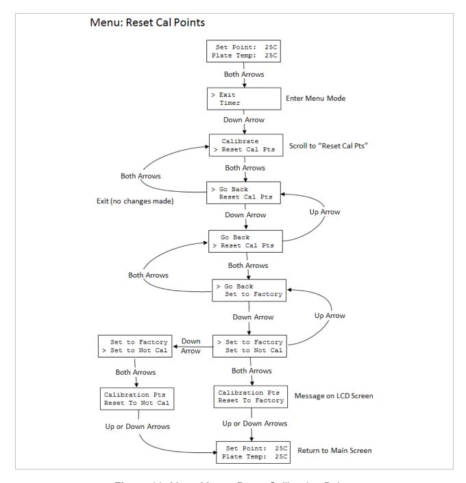
Figure 11: Menu Map to Reset Calibration Points
