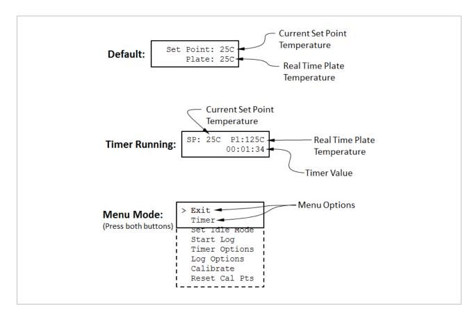
Figure 1: Display Screens for Different Modes of Operation
