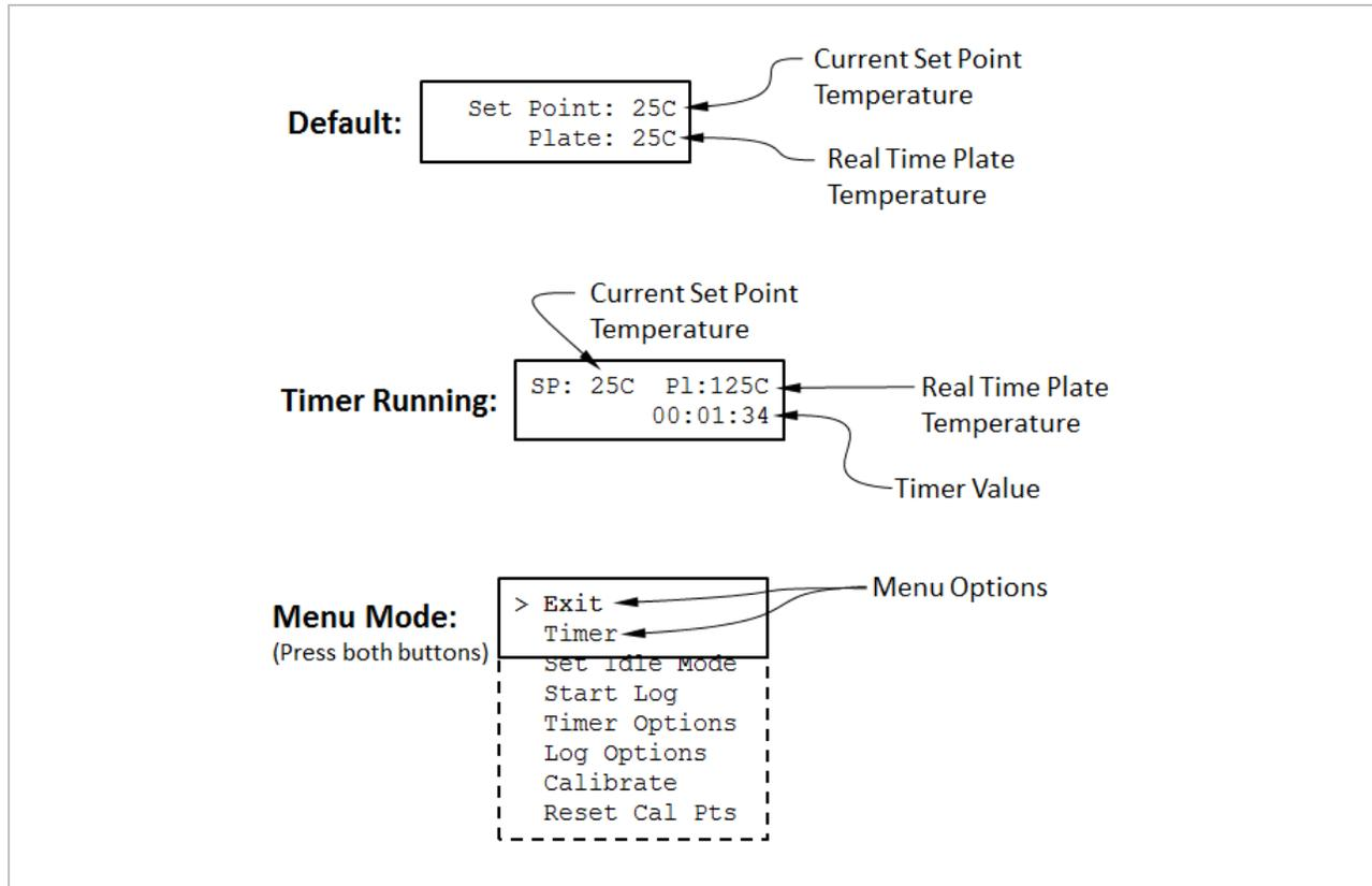
**Figure 1:** Display Screens for Different Modes of Operation
