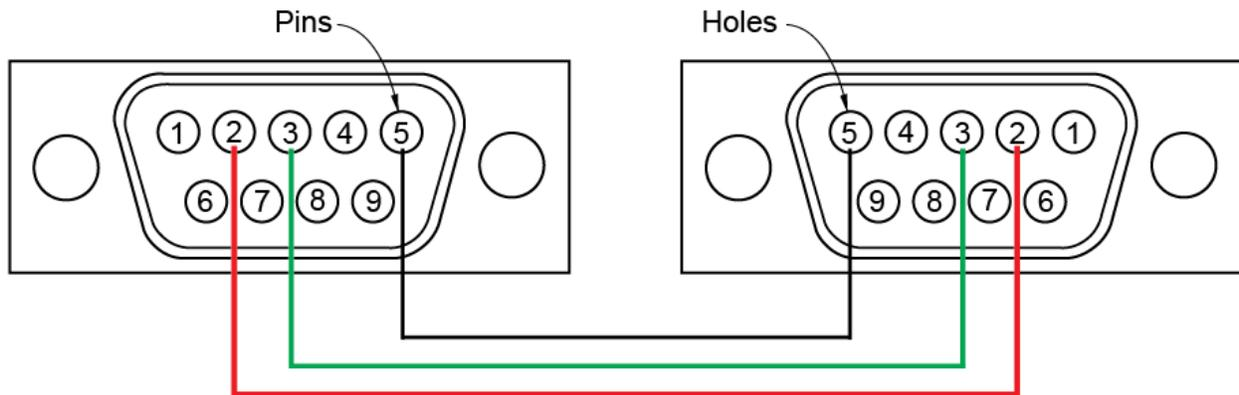
**Figure 12:** RS232 DB9 “Straight Through” Cable Pinout (Pins 2,3,5 only)
