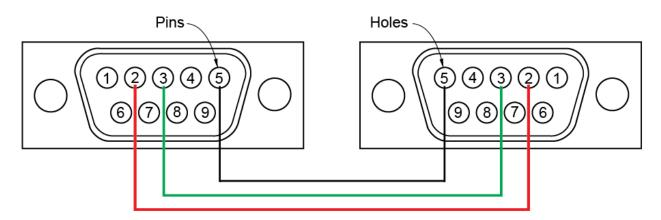
Figure 12: RS232 DB9 "Straight Through" Cable Pinout (Pins 2,3,5 only)
