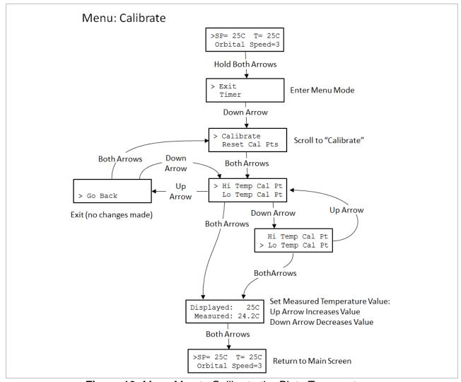
**Figure 10:** Menu Map to Calibrate the Plate Temperatures
