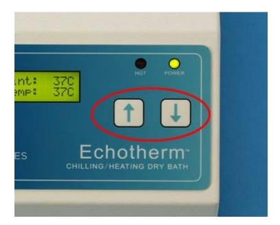
Two push buttons are provided on the front of the unit for user input. One button is labeled with an UP ARROW and the other with a DOWN ARROW. When the buttons are pressed, an audible beep will occur. The keys also have tactile feedback when they are depressed. Using the buttons to set all of the parameters of the unit is accomplished via single and double key presses.
