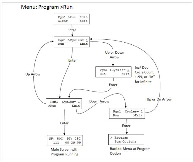
Figure 13: Menu Map For Setting Program Cycles and Running Program
