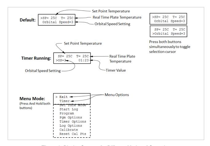
Figure 1: Display Screens for Different Modes of Operation
