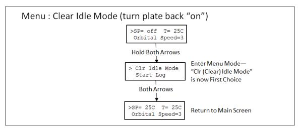
Figure 6: Menu Map to Clear Idle Mode Using the Menu
