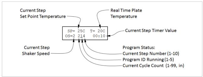
Figure 14: Description of the Display While a Program is Running
