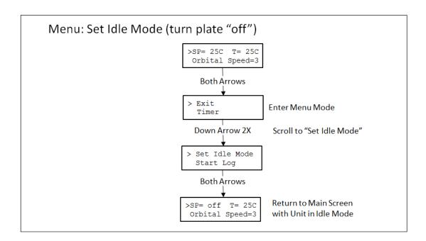
Figure 5: Menu Map to Set Idle Mode Using the Menu
