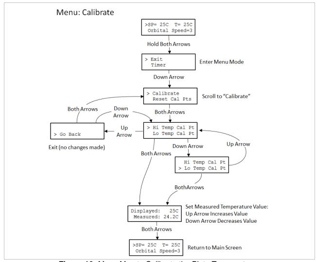
Figure 16: Menu Map to Calibrate the Plate Temperatures
