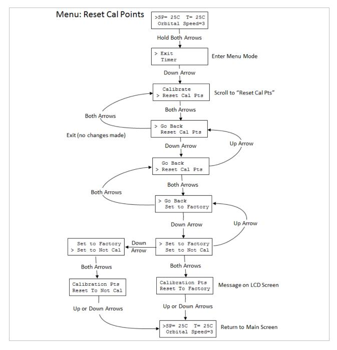
Figure 17: Menu Map to Reset Calibration Points
