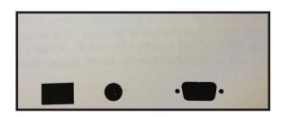
The rear panel shown above has the on/off power switch at the left, the 12 volt dc power input jack in the middle and the RS232 I/O port on the right.
