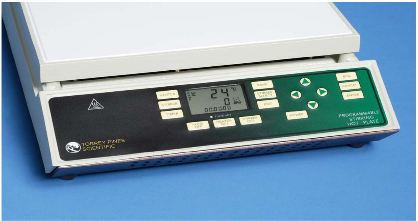
Shown above are the keyboard and display for the HS65 Programmable Digital Hot Plate/Stirrer. This unit has 5-stirring positions and is the most complex unit in the series. Other models in the series will have a single stirring position or no stirrer at all. The keypads will vary depending upon the keys needed for the units in this series with less functions.
