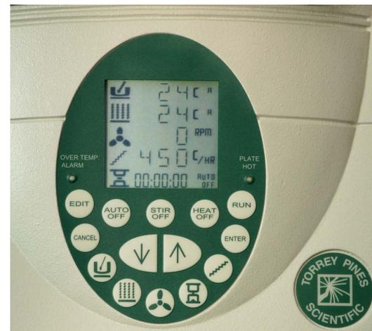
Shown above are the keyboard and display for the HS40 Programmable Digital Hot Plate/Stirrer. **(Note: The hot plate only models will not have the stirrer or stirrer off icons).**
