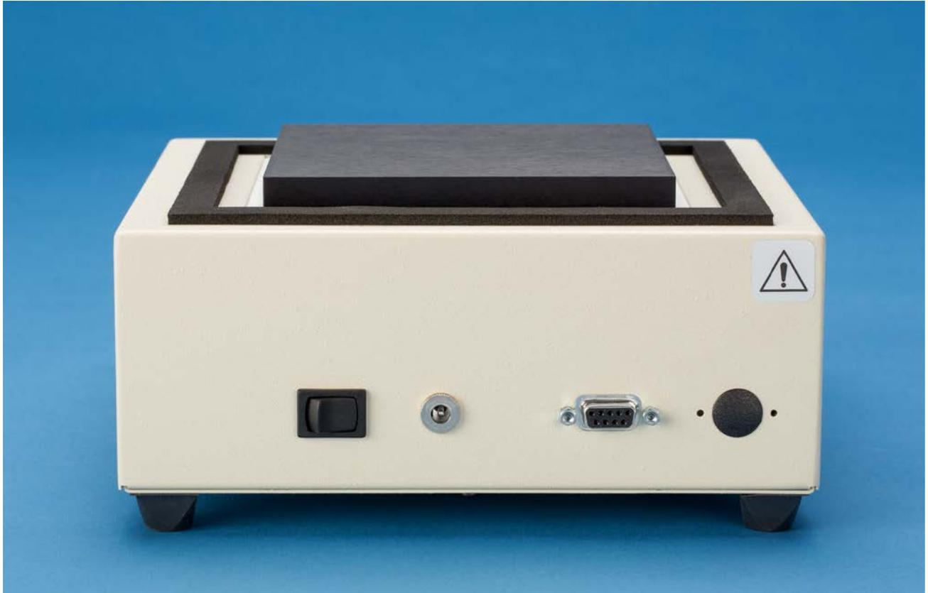
The rear panel shown has the on/off power switch at the left, the 12 volt dc power input jack in the middle, the DB9 connector for the RS232 I/O port is on the right.
